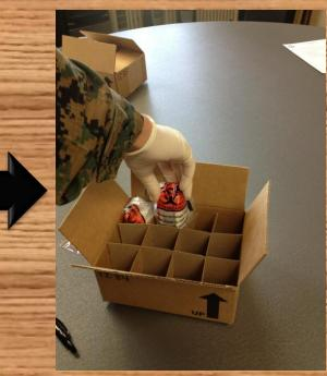
Place each sample to be tested in a waterproof bag Seal the bag and place each bottle in the correct position in the box
